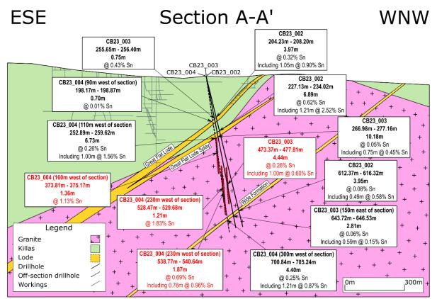
Figure 2. Section A-A' (looking west) of drillholes CB23\_002, CB23\_003 and CB23\_004. Intercepts from the Great Flat Lode, Great Flat Lode Splay, and Wide Formation shown in black. New steeply dipping high-grade tin zones shown in red.
