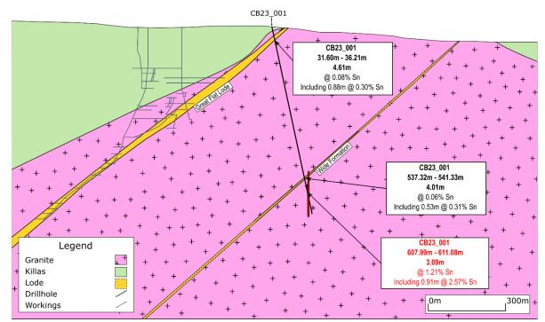
Figure 4. Section C-C' (looking west) of drillhole CB23\_001. Intercepts from the Great Flat Lode and Wide Formation shown in black. New steeply dipping high-grade tin zones shown in red.
