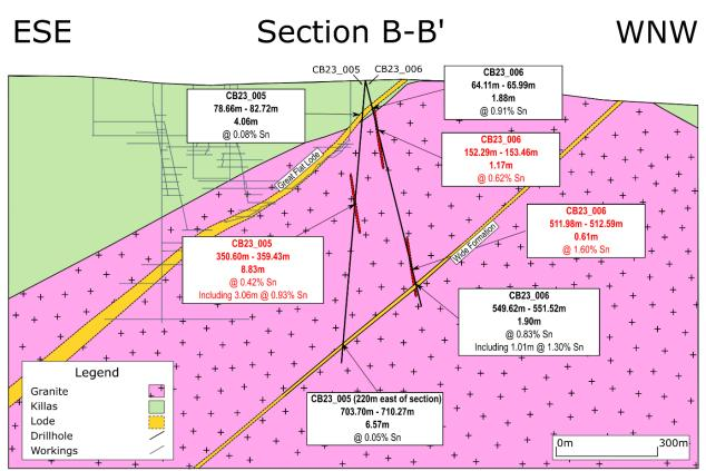
Figure 3. Section B-B' (looking west) of drillholes CB23\_005 and CB23\_006. Intercepts from the Great Flat Lode and Wide Formation shown in black. New steeply dipping high-grade tin zones shown in red.
